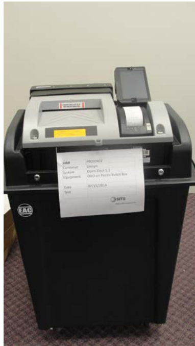
Figure 1-1 OVO on Plastic Ballot Box
