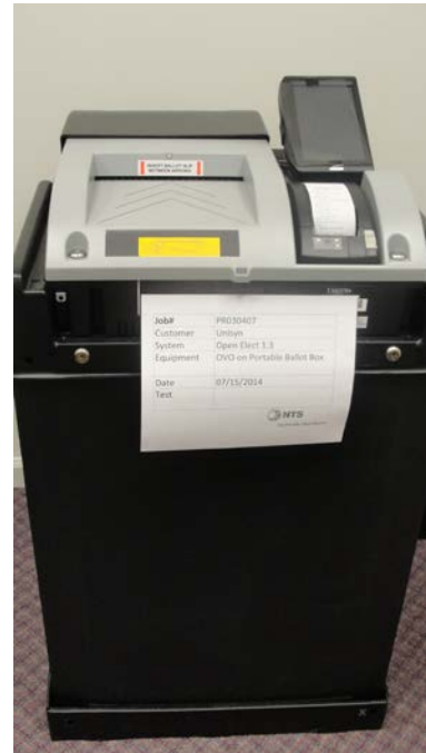
Figure 1-2 OVO on Portable Ballot Box
