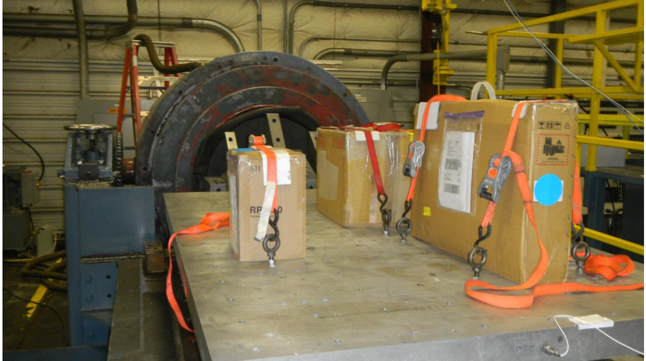
Photograph 7 Vibration – Longitudinal Axis
