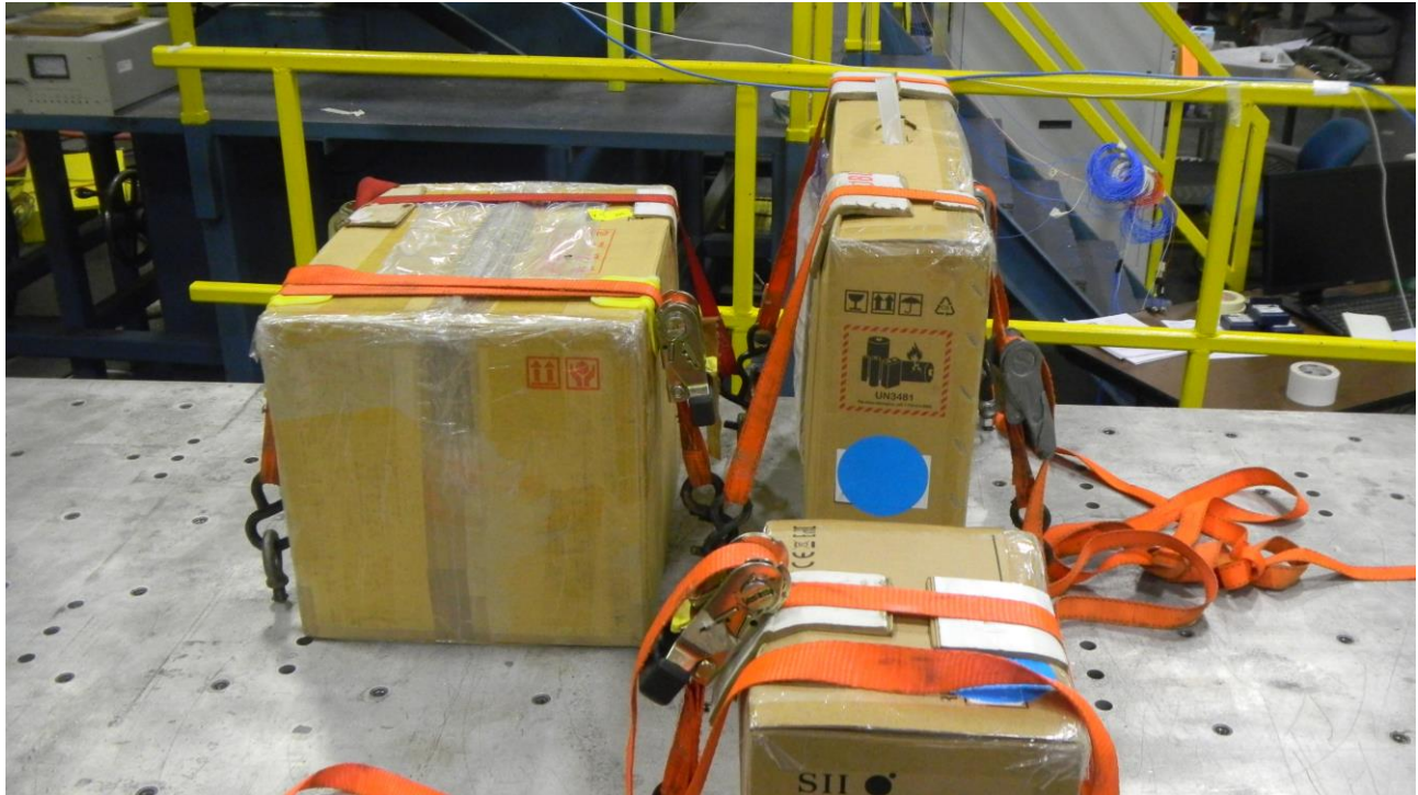
Photograph 6 Vibration – Transverse Axis
