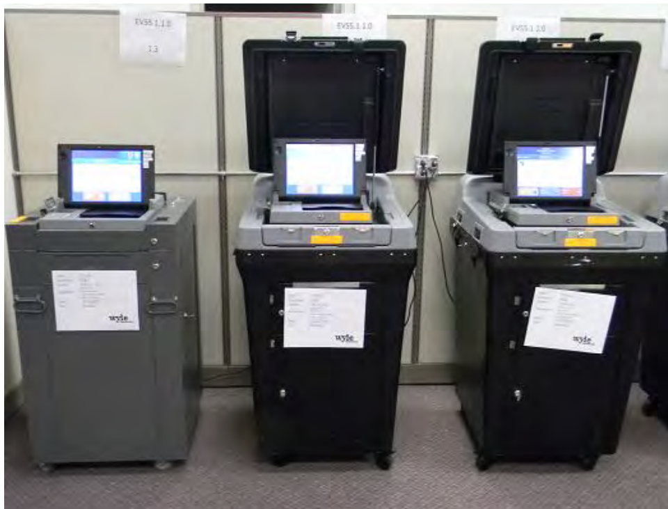
Photograph No. 2 ES&S EVS 5.0.1.0 Accuracy Test Setup
