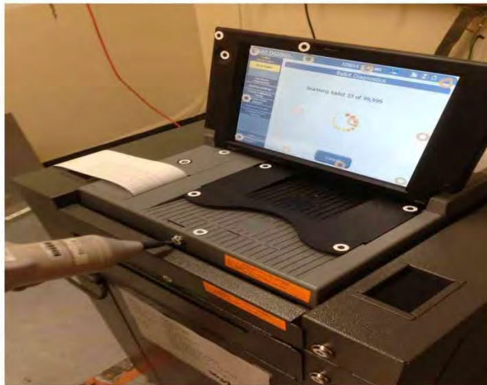
Photograph 18: ES&S FL EVS 4.5.0.0 Electrostatic Disruption
