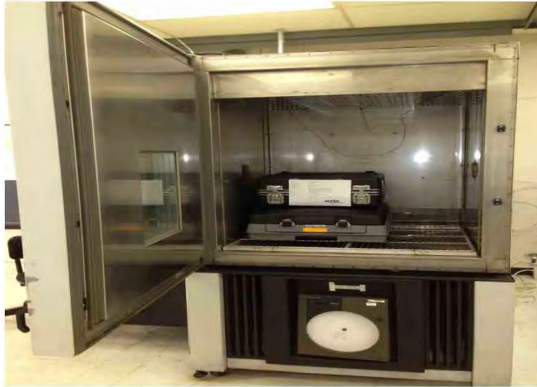
Photograph 31: ES&S FL EVS 4.5.0.0 High Temperature
