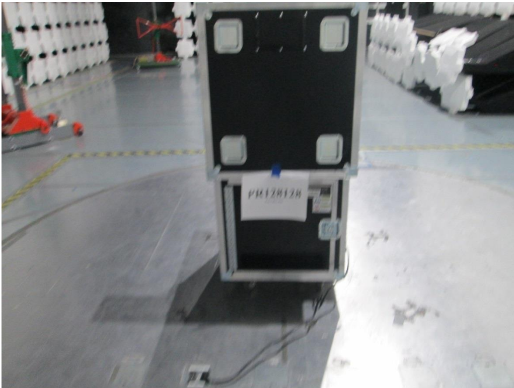
Figure A4: Radiated Emissions Test Setup – Back Side
