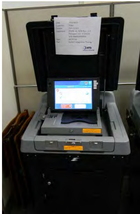
Photograph No. 12 DS200 System Integration Test Setup
