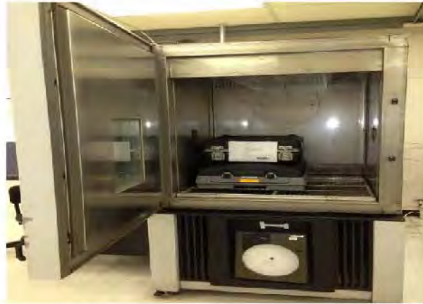
Photograph 31: ES&S FL EVS 4.5.0.0 High Temperature
