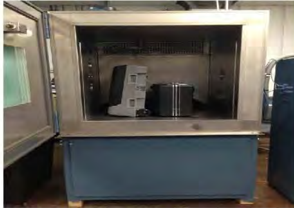
Photograph 29: ES&S FL EVS 4.5.0.0 Low Temperature
