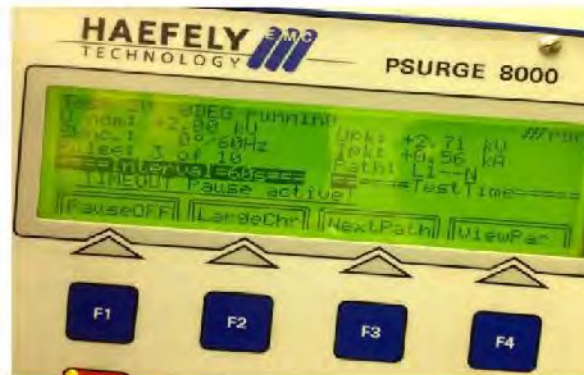
Photograph 11: ES&S FL EVS 4.5.0.0 Lightning Surge
