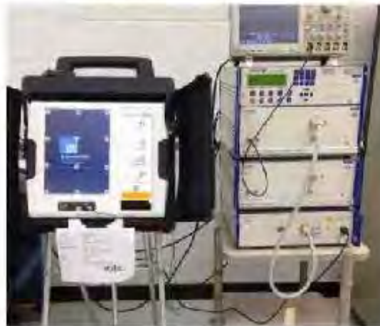
Photograph No. 12: ES&S BL ENS 4.50.01 lightning Surge
