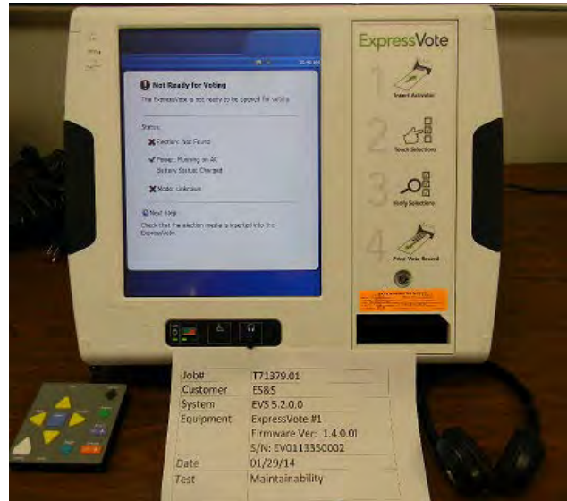
Photograph No. 5 ExpressVote Maintainability Test Setup
