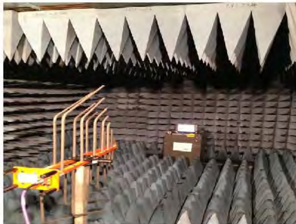
Photograph 22: ES&S FL EVS 4.5.0.0 Electromagnetic Susceptibility
