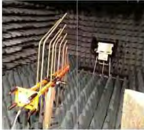
Photograph No. 23: ES&S FL EVS 4.5.0.0 Electromagnetic Susceptibility
