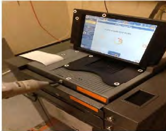
Photograph 18: ES&S FL EVS 4.5.0.0 Electrostatic Disruption
