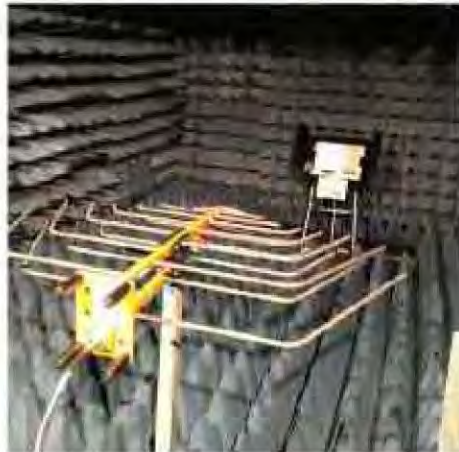
Photograph No. 24: ES&S FL EVS 4.5.0.0 Electromagnetic Susceptibility
