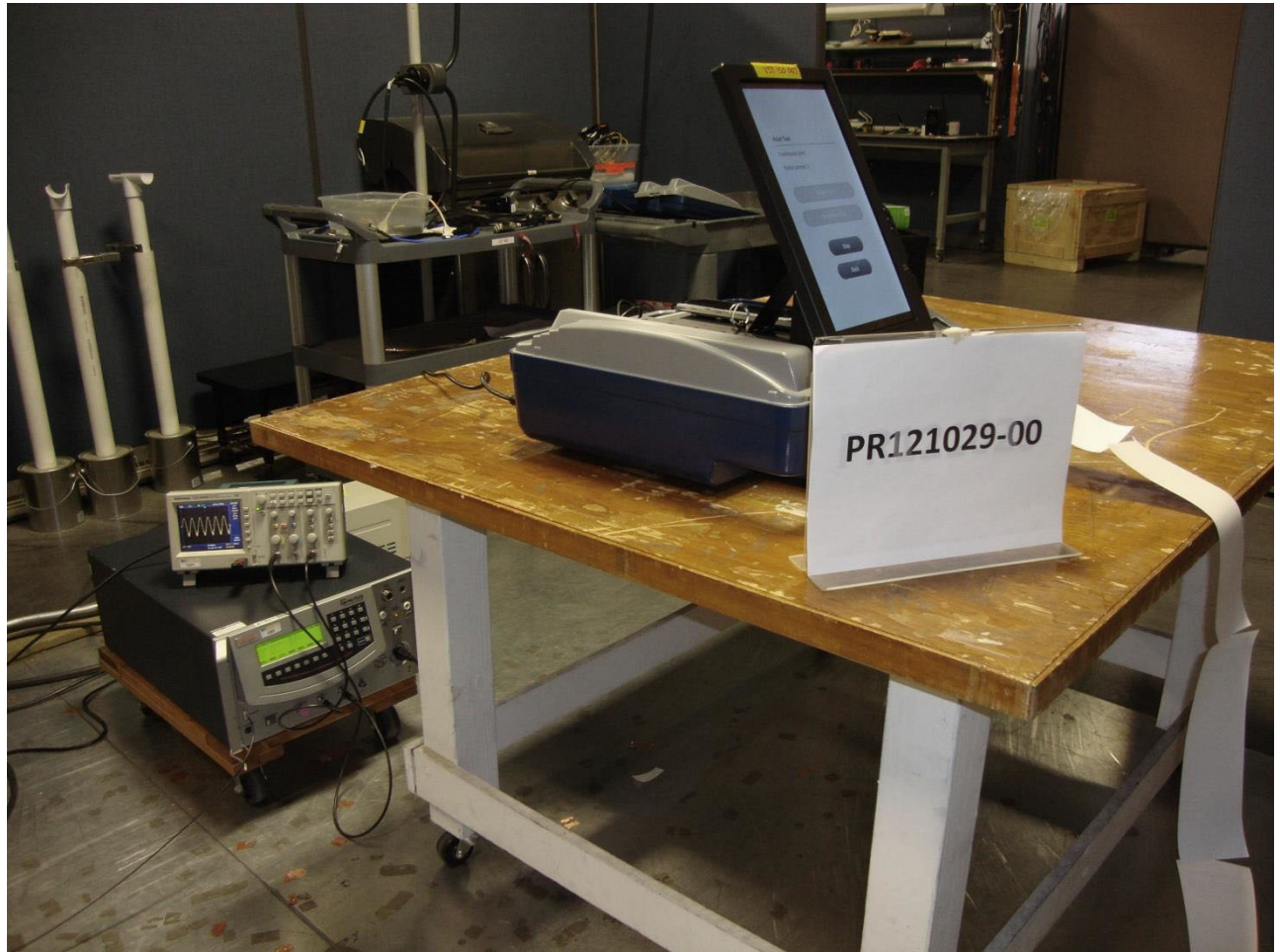
Figure D1. Surge Immunity Test Setup.
