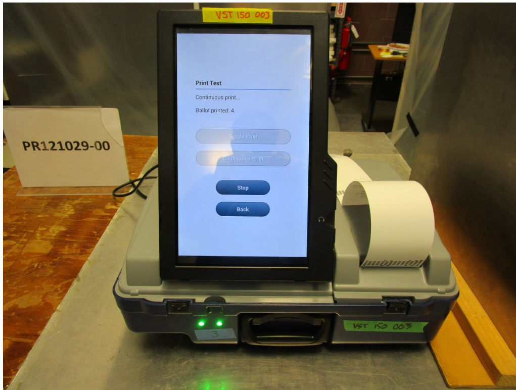
Figure A2. Electrostatic Discharge Test Setup.
