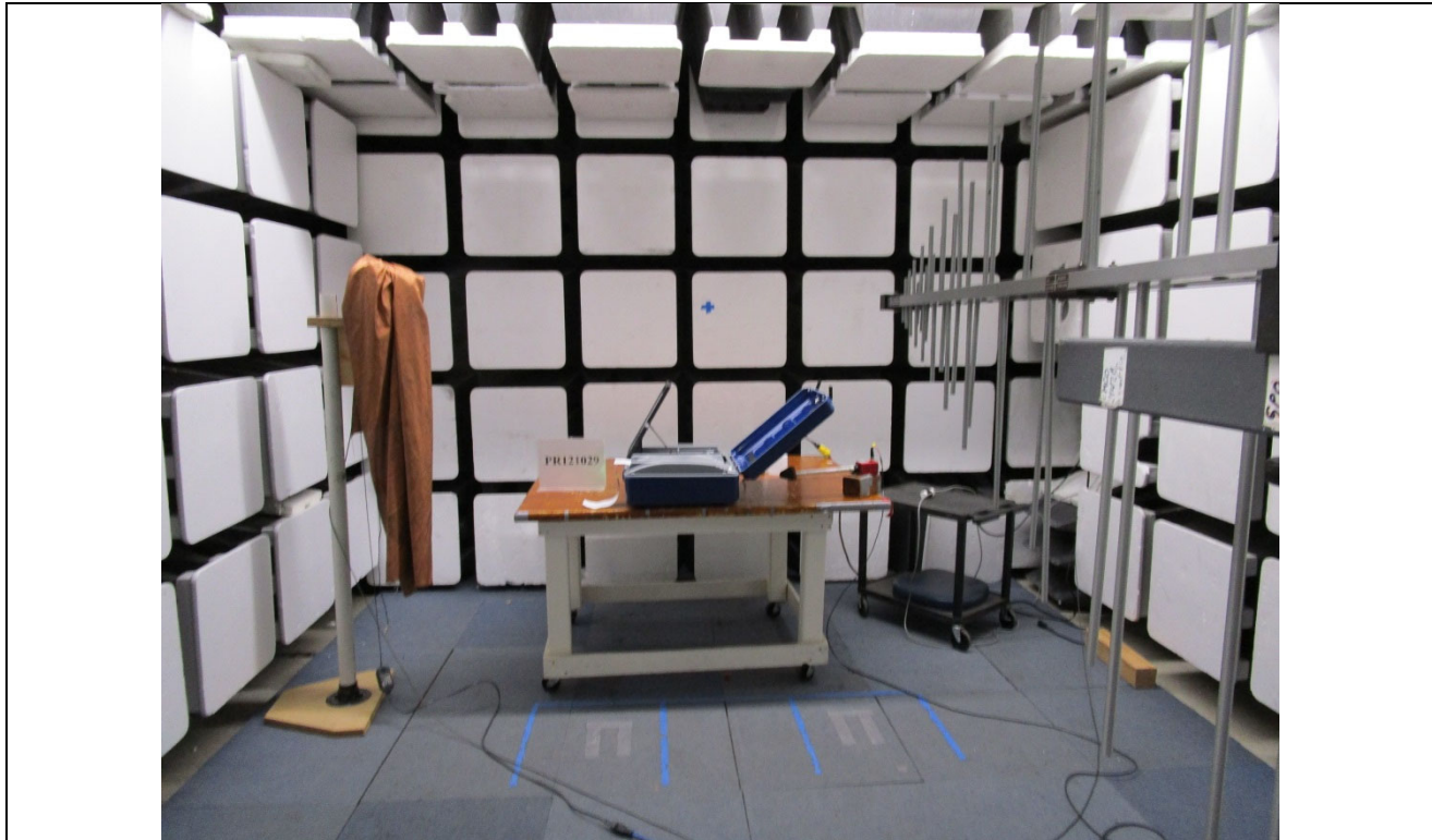
Figure B2. Radiated RF Immunity Test Setup – Right Side.
