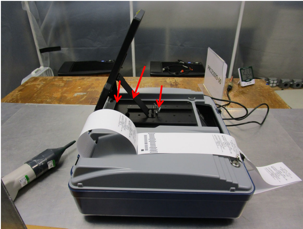
Figure A3. Electrostatic Discharge Test Setup.
