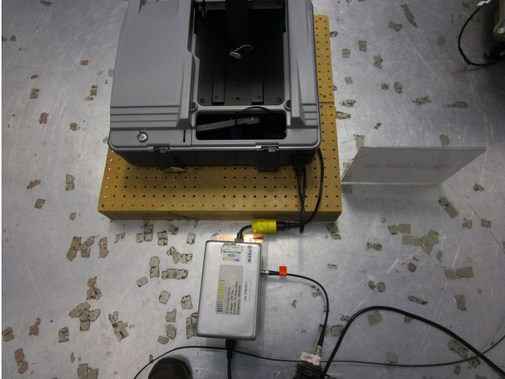
Figure E2. Conducted RF Immunity Test Setup – AC Mains.
