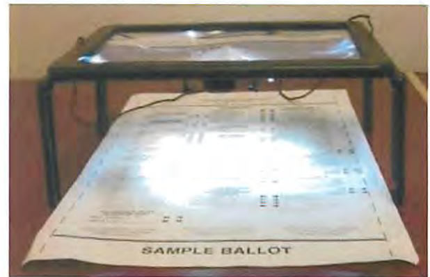
FIGURE 7 COMMERCIALY AVAILABLE STANDOFF MAGNIFIER: UNSTABLE, HIGH GLARE, UNEVEN ILLUMINATION.
